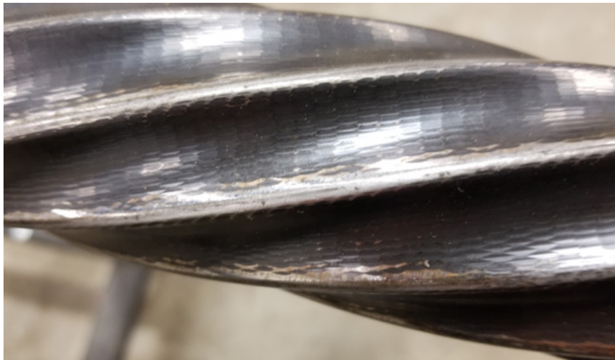
Figure 3 - Alternate view of rotor contact patch
