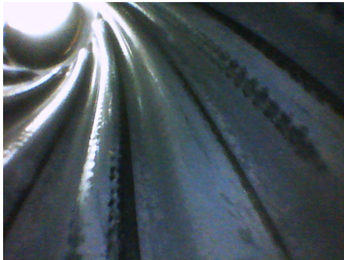
Figure 4 - Post-run borescope of stator
