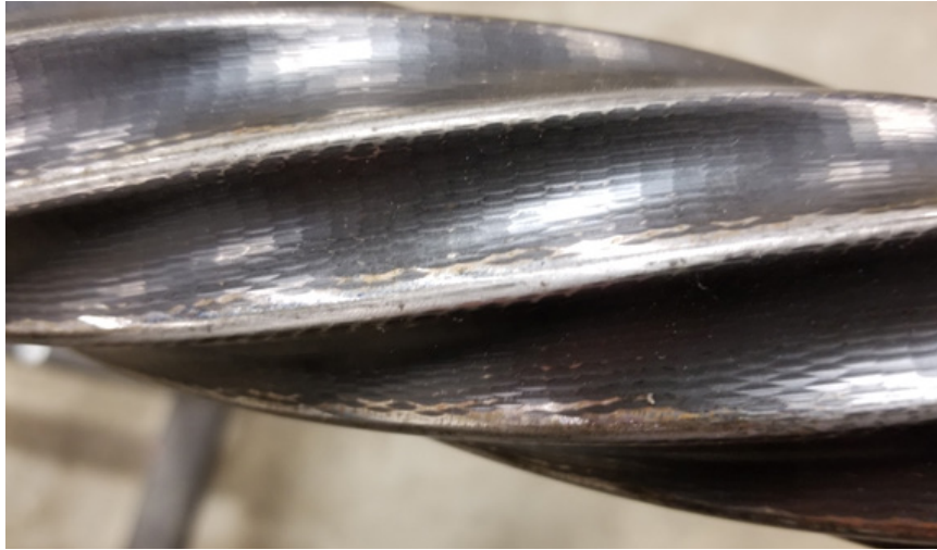
Figure 2 - Closeup of rotor contact patch
